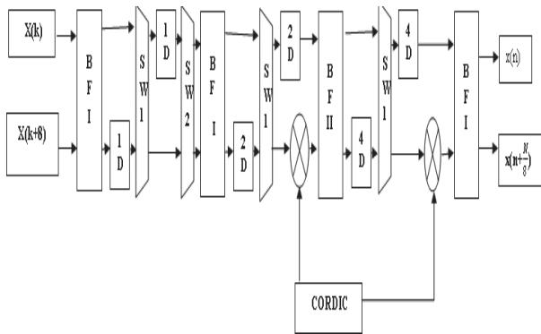
Fig. 10 Proposed Modified Scaling-Free CORDIC based two-parallel pipelined MDC architecture for a radix-2<sup>2</sup> 16-point IFFT
