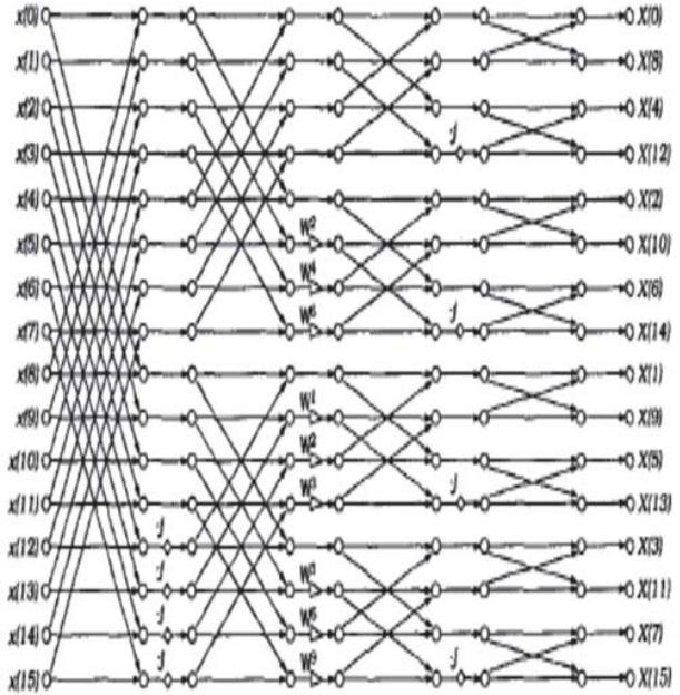
Fig. 1 Flow graph of a radix-2<sup>2</sup> 16-point DIF FFT
