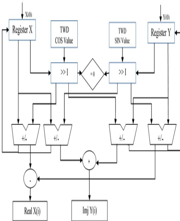
Fig. 9 Modified Scaling free CORDIC based Complex Multiplier
