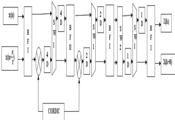
Fig. 2 Proposed Modified Scaling-Free CORDIC based two-parallel pipelined MDC architecture for a radix-2<sup>2</sup> 16-point FFT
