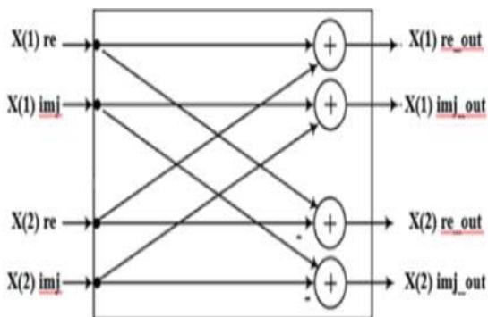
Fig. 3 Structure of the Butterfly Unit I
