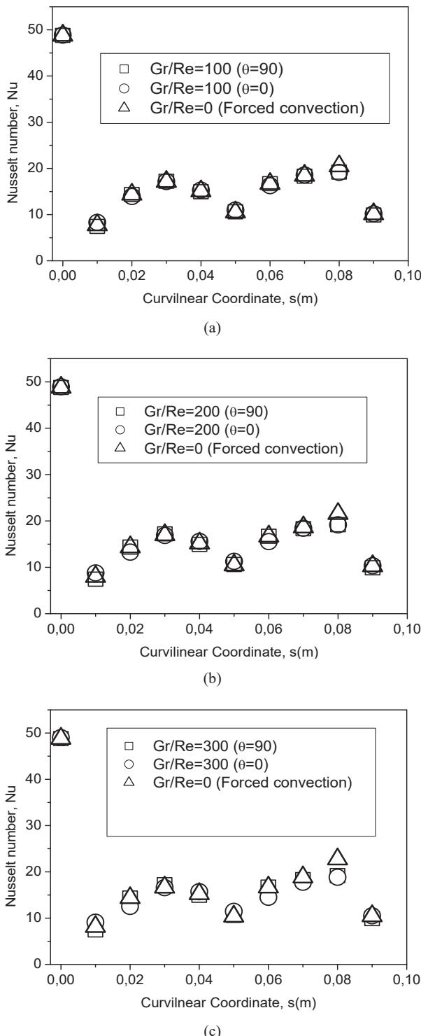
Fig. 3 Evolutions of the Nusselt number,  $Nu$ , versus the curvilinear coordinate, (a)  $Gr/Re = 100$ , (b)  $Gr/Re = 200$ , and (c)  $Gr/Re = 300$ .
