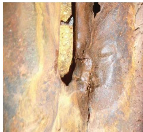
Fig. 1 Cracks at fin tip of tubes membrane
