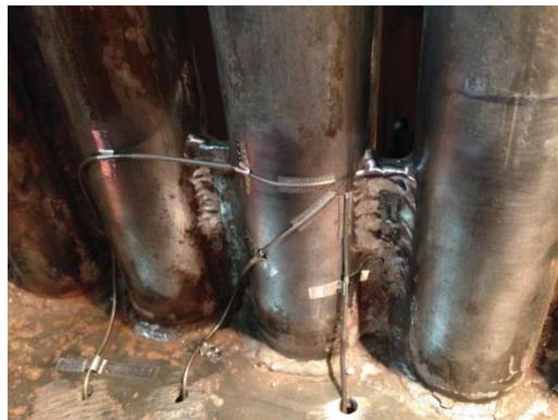
Fig. 3 Strain gage installation on boiler tubes
