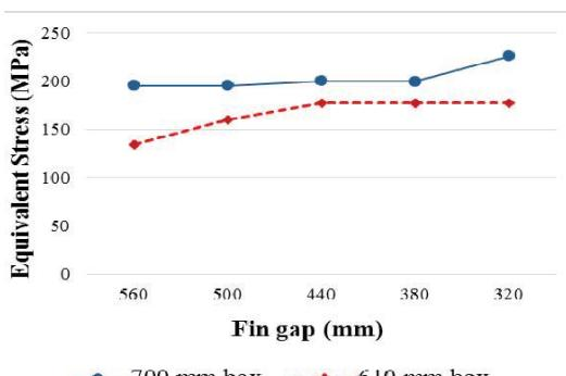
Fig. 14 Relationship between fin gap and equivalent stress
