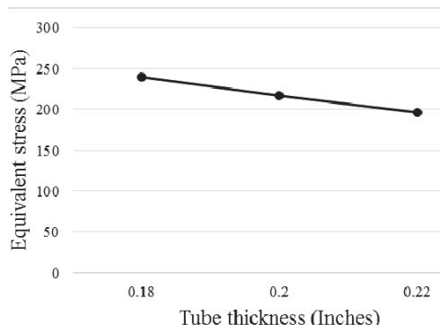
Fig. 12 Relationship between tube thickness and equivalent stress
