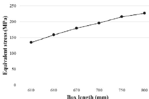
Fig. 13 Relationship between box length and equivalent stress
