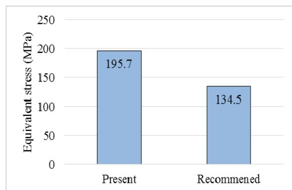
Fig. 15 Comparison of equivalent stress between two designs
