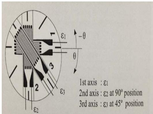
Fig. 4 Strain gages in 45°-rectangular rosette orientation
