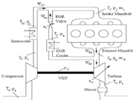
Fig. 1 Air path of modern diesel engine [7]
