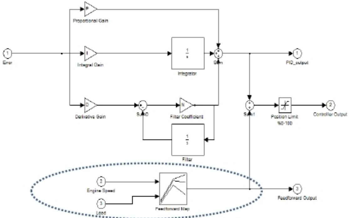
Fig. 9 PID+open loop feed-forward control
