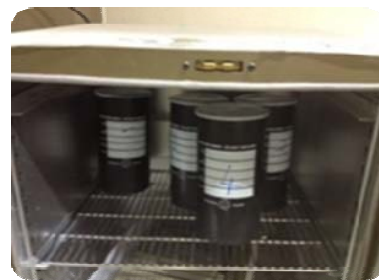
Fig. 7 Storage of mortar bars for AMBT test
