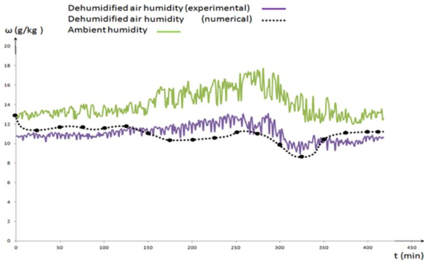
Fig. 7 Variation of numerical and experimental dehumidified air humidity
