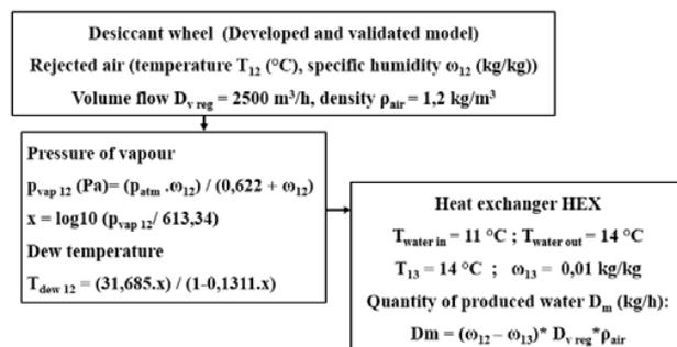
Fig. 14 Calculation procedure for the water condensation compartment
