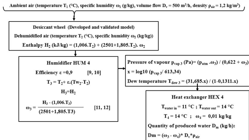
Fig. 10 Calculation procedure for the desalination compartment
