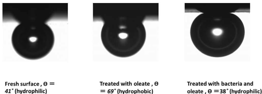
Fig. 7 Contact angle of dolomite under different conditions
