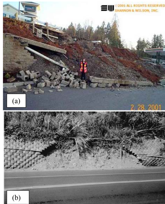
Fig. 1 Collapsed Reinforced Earth Walls During Earthquakes. (a) Extended Stay Hotel MSE Wall-Seattle collapsed after the Nisqually earthquake (USA-PEER 2001), (b) Collapsed Wall at Highway 129 after Chi Chi Earthquake [5]
