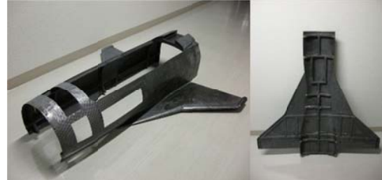
Fig. 14 Full composite semi-monocoque structure of WIRES#014
