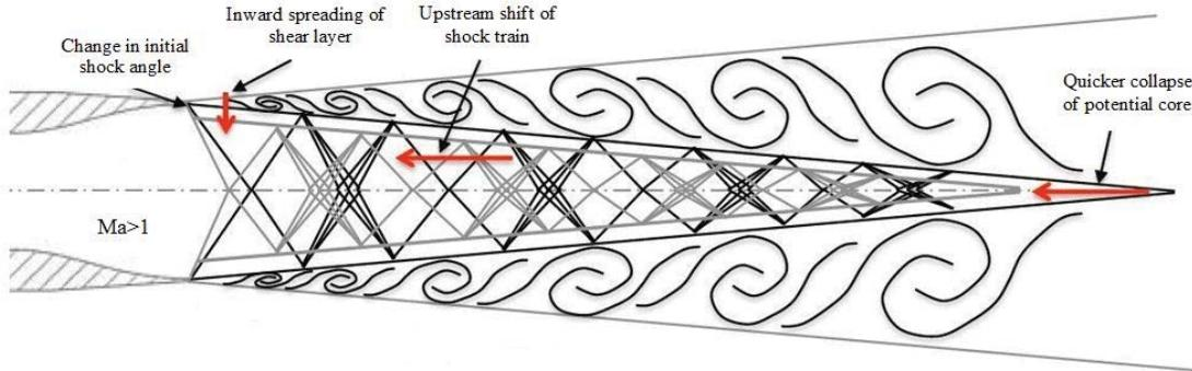
Fig. 1 Schematic of the structure of fluidic injection [15]
