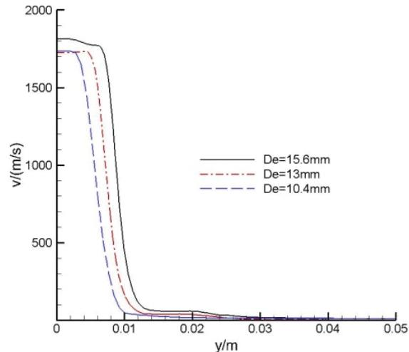
Fig. 8 Velocity distribution along the radial at  $x=0.2$ m
