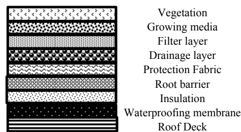
Fig. 1 Structure of green roof system
