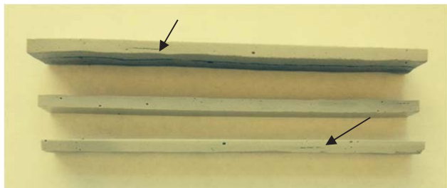
Fig. 7 DMA specimens from polyester composite after eight months exposure to water at 40°C for eight months
