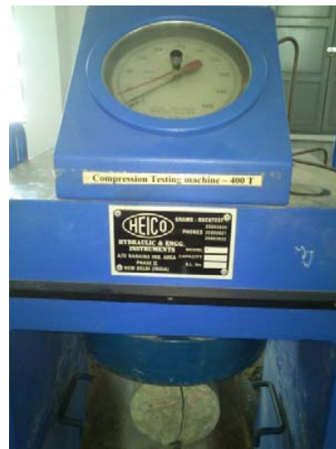
Fig. 10 Split Tensile strength Test
