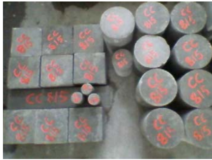
Fig. 5 Casting of Cubes
