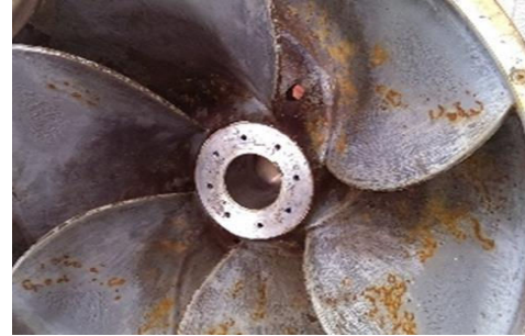
Fig. 16 Cavitation of Impeller
