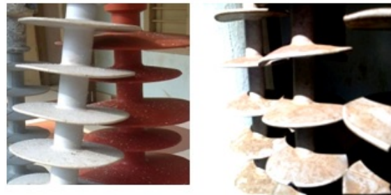
Fig. 8 33 kV Specimens under salt pollution
