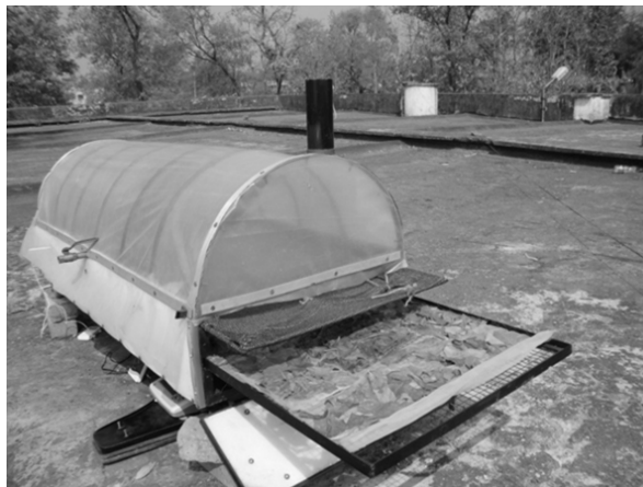
Fig. 1 Experimental set-up of spinach drying in solar tunnel dryer (STD)
