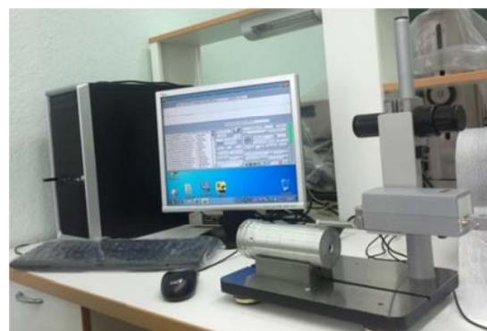
Fig. 3 Measuring surface roughness using profilometer model 130
