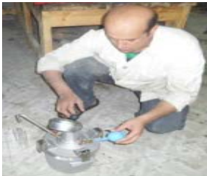
Fig. 4 Air content for fresh geopolymer concrete
