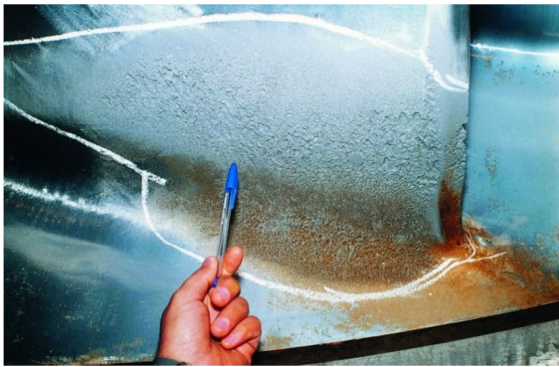
Fig. 1 Cavitation damage on runner blade surface
