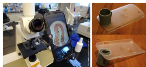
Fig. 6 Adapters of smartphone for taking microscopic pictures, they are commercial (A) or hand-made (B) adapters. They can be fixed on the eyepiece or on the stage of the light microscope
