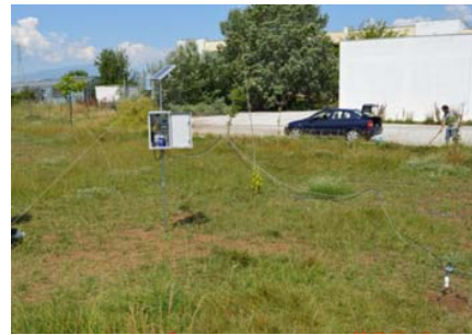
Fig. 4 The field setup of the Automated Soil Erosion Monitoring System (ASEMS)
