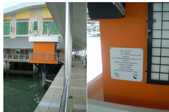
Fig. 4 JUPEM-automated tide gauge at Kukup Port
