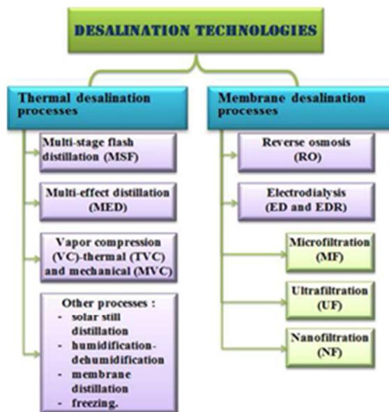
Fig. 1 Classification of desalination technologies [7]
