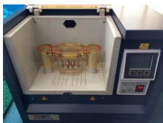
Fig. 3 Bispherical electrode system for measurement of breakdown voltage
