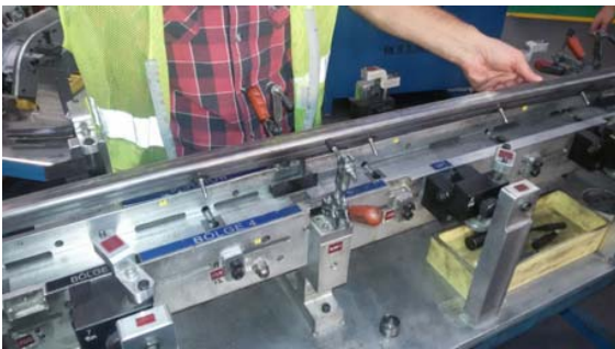
Fig. 10 Fixture Measured After the Stud Welding
