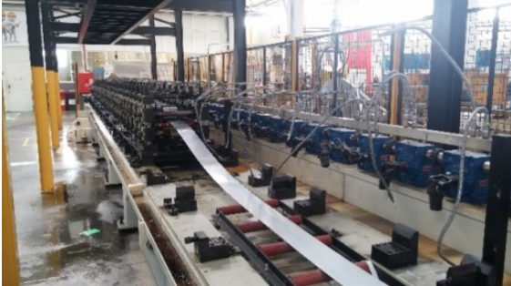
Fig. 5 Forming Sheet Work Piece in Roll-form Line
