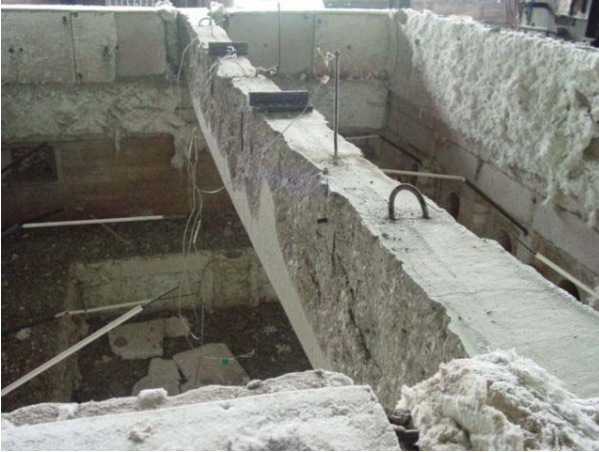
Fig. 6 Specimen on the horizontal heating furnace after fire test
