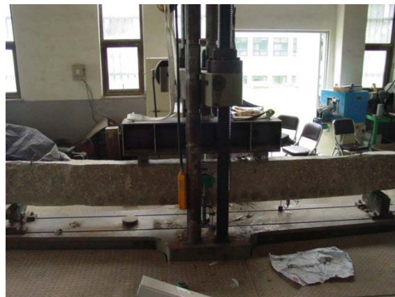
Fig. 5 Four-point loading test of rehabilitated beam
