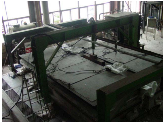
Fig. 4 The horizontal heating furnace for fire test
