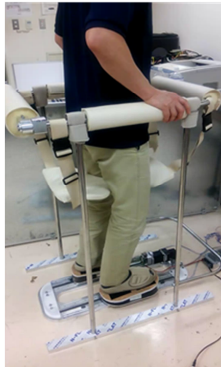
Fig. 3 The training robot for the basic walking pattern for home use. The robot has simplified functions and mechanisms, and a robust and easy to use user interface. The light weight, low cost and safety are important for the home use
