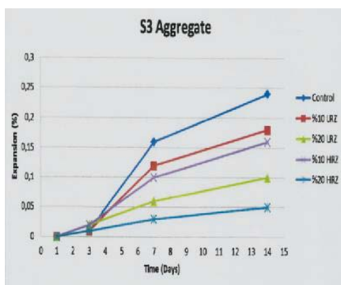
Fig. 4 Expansions of mortar bars cast with S3 aggregate
