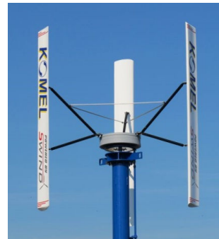
Fig. 8 VAWT wind plant with Komel's generator
