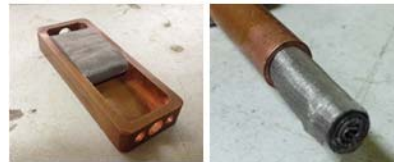
Fig. 4 Stainless steel screen mesh capillary wick
