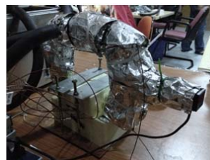
Fig. 6 Flat plate loop heat pipe assembly.
