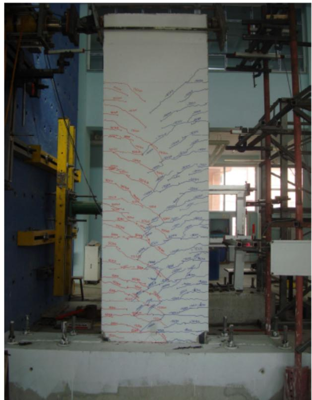
Fig. 9 Cracking patterns of CSW at failure stage
