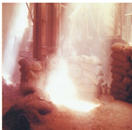
Fig. 2 Dust emissions from paddy Silo
