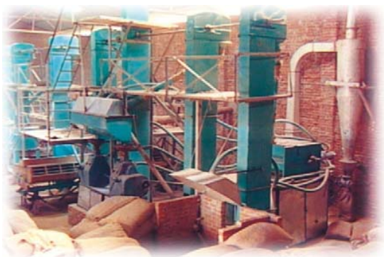
Fig. 7 Rice Sheller along with integrated APCD
