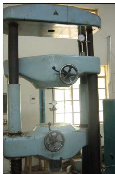
Fig. 3 Pull out Test
