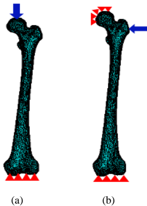
Fig. 2 Application of loading and boundary conditions during (a) the single-leg stance, and (b) the sideways fall
