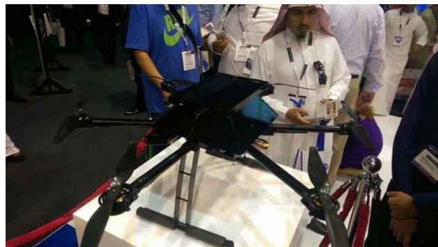
Fig. 4 The UAV, equipped with a Kinect and a Surface Pro device, will not only carry a tube but be able to detect individuals in distress and deliver the tube [6]
