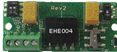
Fig. 6 Buck boost circuitry as power electronics circuit
