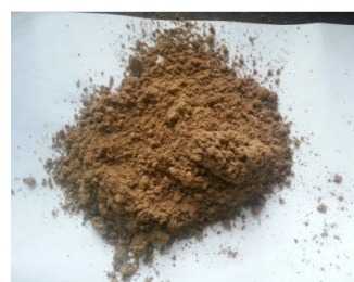
Fig. 1 Groundnut shell particulate
