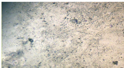
Fig. 19 Micrograph of 15% cow bone filler
