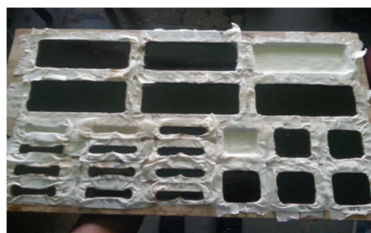
Fig. 3 Mould filled with GSRPC samples
