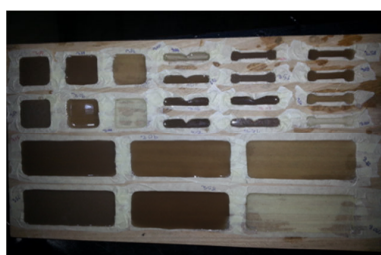
Fig. 5 Mould filled with HRPC samples
