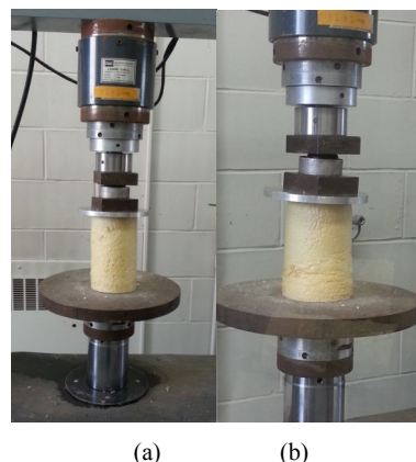
Fig. 3 Compression test on LPF samples, (a) before loading, (b) after loading
