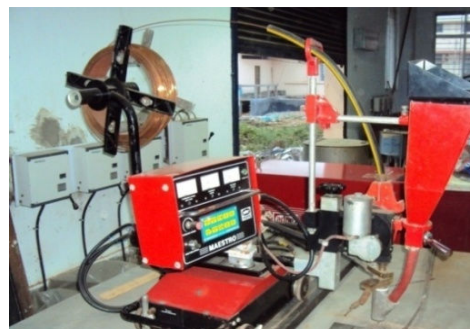
Fig. 1 Photographic view of SAW unit
