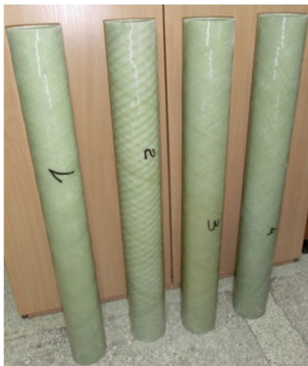
Fig. 2 Prepared composite samples before testing
