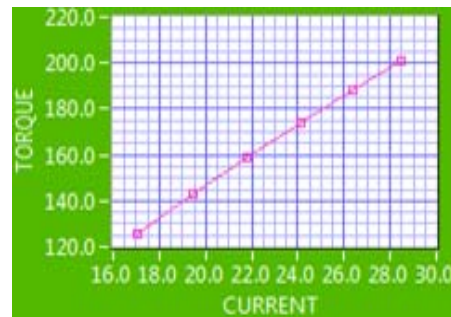
Fig. 5 Torque vs current characteristics of induction motor
