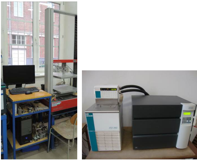
Fig. 4 Apparatus for determine of mechanical and thermal insulating properties
