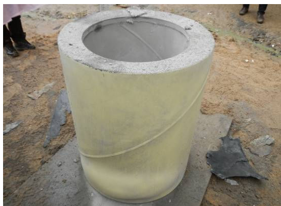
Fig. 8 Litter bin after real blast test
