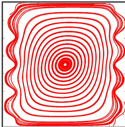
Fig. 5 Streamlines for Ra- $10^4$  for Rough Cavity
