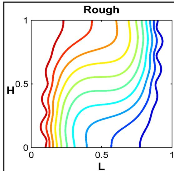
Fig. 9 Isotherms for Ra- $10^4$  for Rough Cavity
