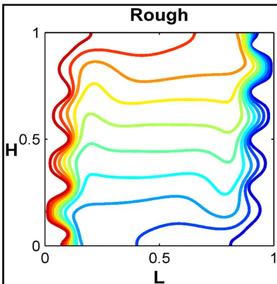
Fig. 11 Isotherms for Ra-106 for Rough Cavity
