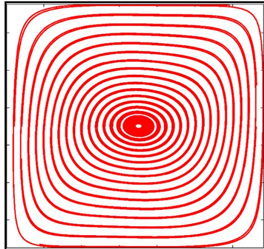
Fig. 4 Streamlines for Ra- $10^4$  for Smooth Cavity
