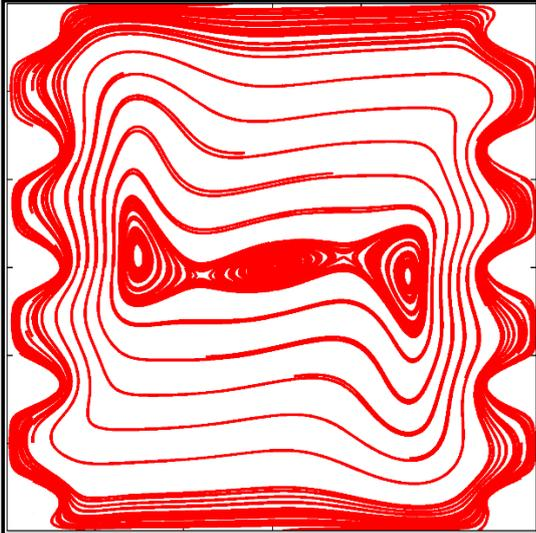
Fig. 7 Streamlines for Ra- $10^6$  for Rough Cavity
