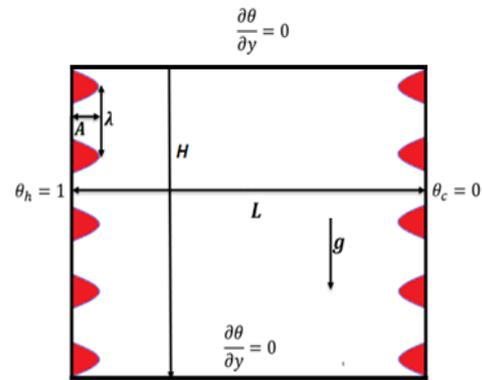
Fig. 1 A Square Cavity with Sinusoidal Roughness
