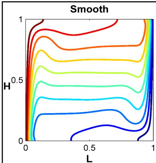
Fig. 10 Isotherms for Ra-106 for Smooth Cavity
