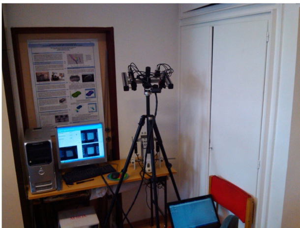
Fig. 7 Combination of VIALUX system & bi-axial stress measuring
