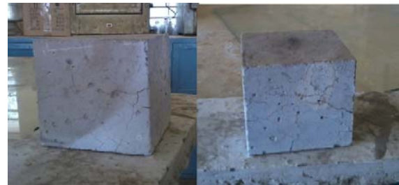
Fig. 3 Concrete specimens subjected to 800°C
