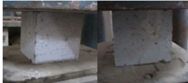
Fig. 2 Concrete specimens subjected to 400°C and 600°C
