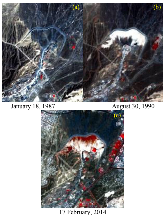
Fig. 5 (a) (c) Landsat data shows the siltation (white) and vegetation (red) in the Alkhod dam
