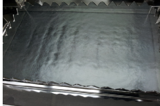
Fig. 1 Uniform cavitation activity in 360 kHz frequency operating in thickness mode transducers
