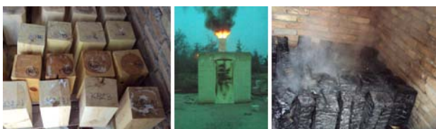
Fig. 2 The image where placements of wooden samples, the moment of fire and after fire exist
