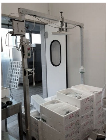
Fig. 6 Boxes with RFID labels and RFID data logger pass the portal
