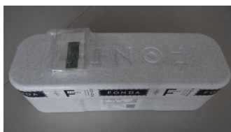
Fig. 4 RFID data logger (SL900A) on a box
